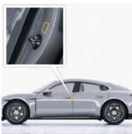
Fig. 216: Safety compliance sticker
