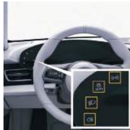
Fig. 96: Light control panel
