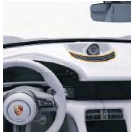
Fig. 21: Upper ventilation panel
