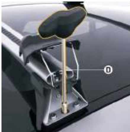
Fig. 146: Tightening the anchoring bolts
