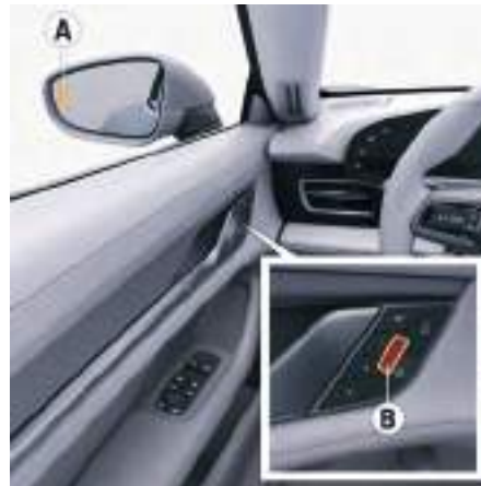
Fig. 66: Exit Warning indicator elements
