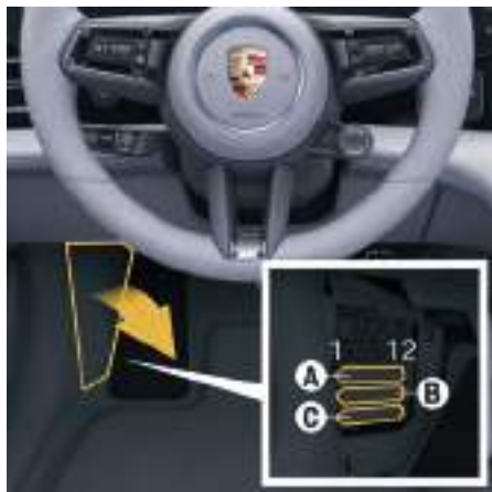
Fig. 70: Opening fuse box in left footwell
