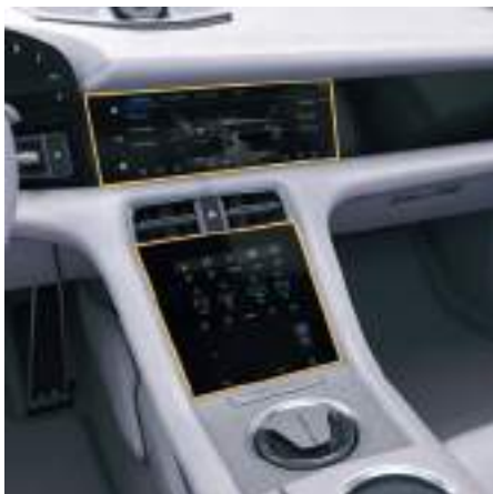
Fig. 4: Air-conditioning control panels
