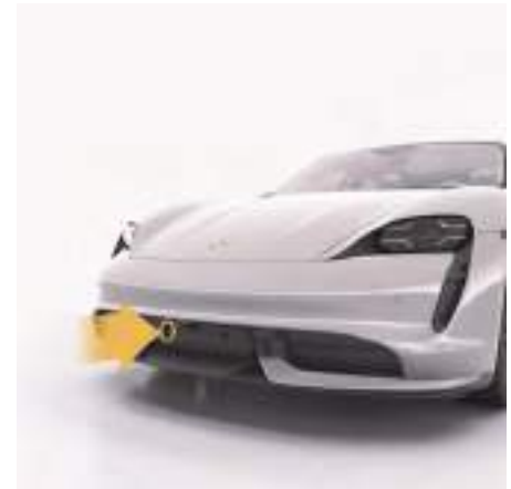
Fig. 129: Radar sensor position
