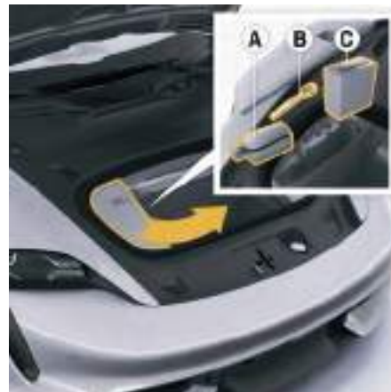
Fig. 101: Plastic box for tire sealant (Tire Mobility System - TMS), towing hook and first aid kit (depending on country)
