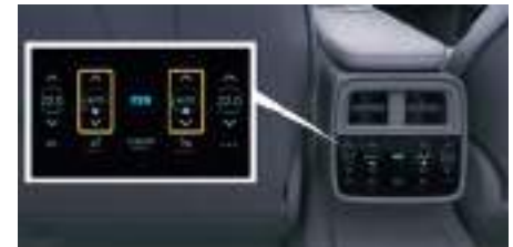
Fig. 25: Setting the air flow in the rear
