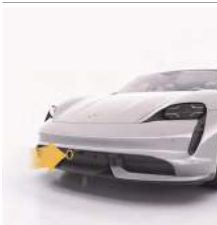
Fig. 8: Radar sensor position
