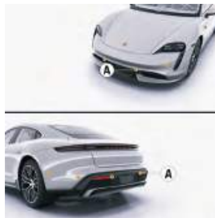
Fig. 114: Ultrasound sensors for distance measurement
