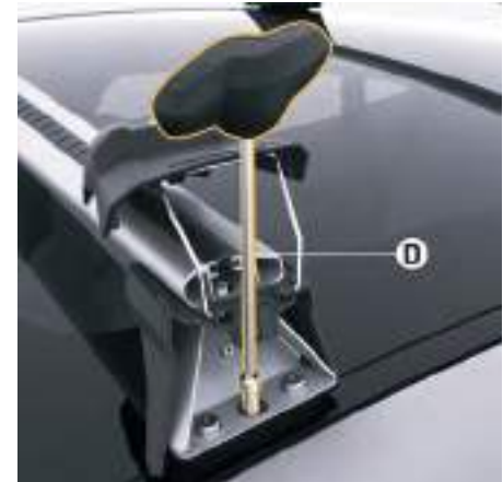
Fig. 150: Tightening the anchoring bolts
