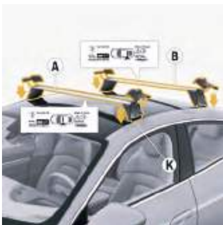
Fig. 145: Placing the carrier on the roof
