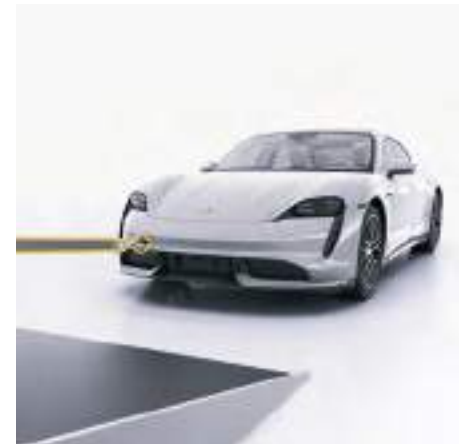
Fig. 187: Pulling vehicle onto flat bed
