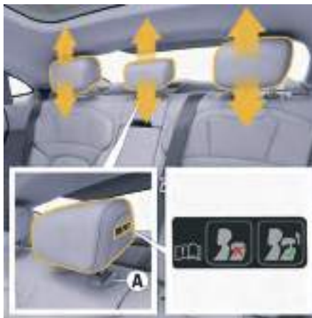
Fig. 163: Adjust the height of the headrests on the rear seats (example: three seats in the back)
