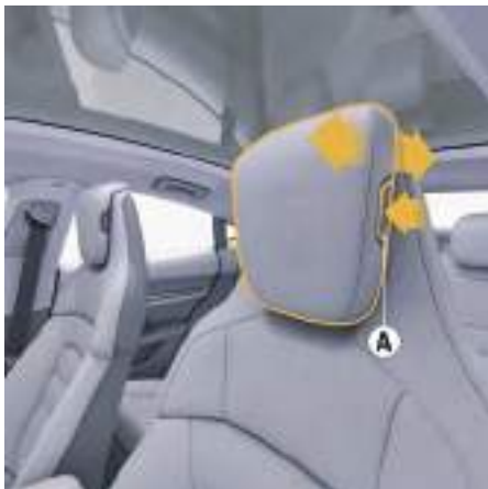
Fig. 162: Adjust the horizontal position of the head rests on the front seats
